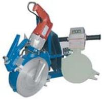
Removable PTFE-coated heating plate with an electronic temperature control.
