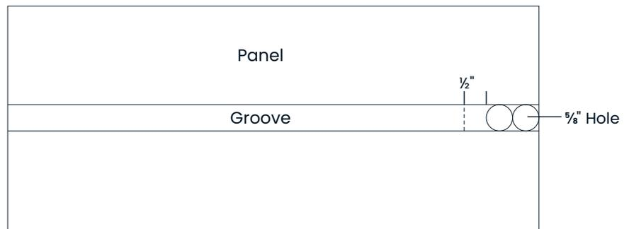
**Figure 24:** Drill two holes to create a rectangular slot in the subfloor.
