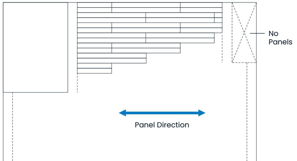
**Figure 18: Stagger panels so seams do not line up.**
