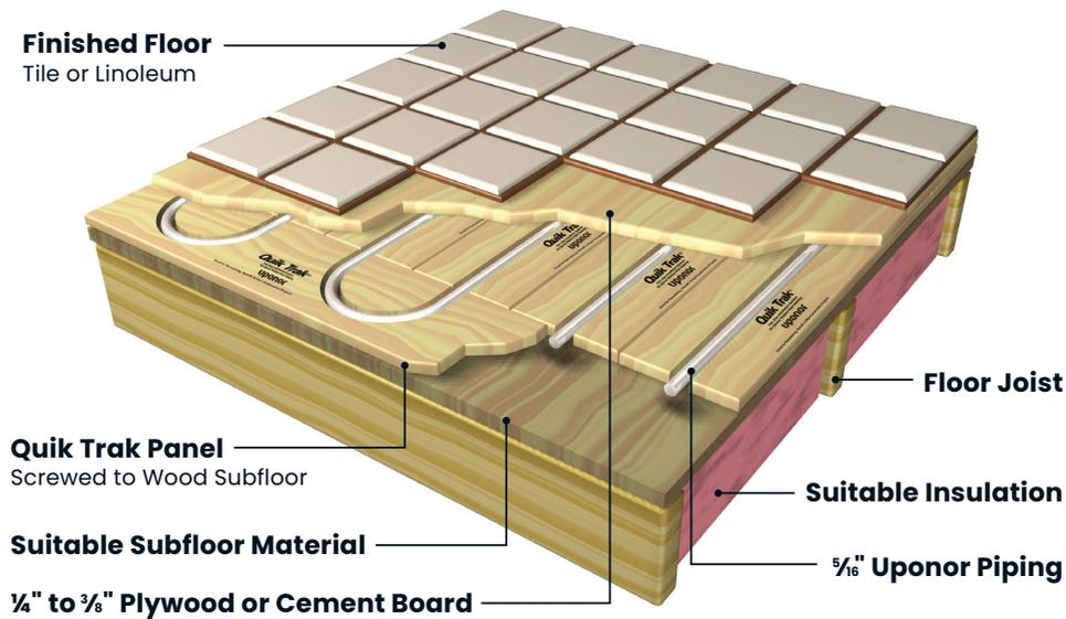
**Figure 5: Quik Trak over a wood subfloor with tile/linoleum floor covering**
