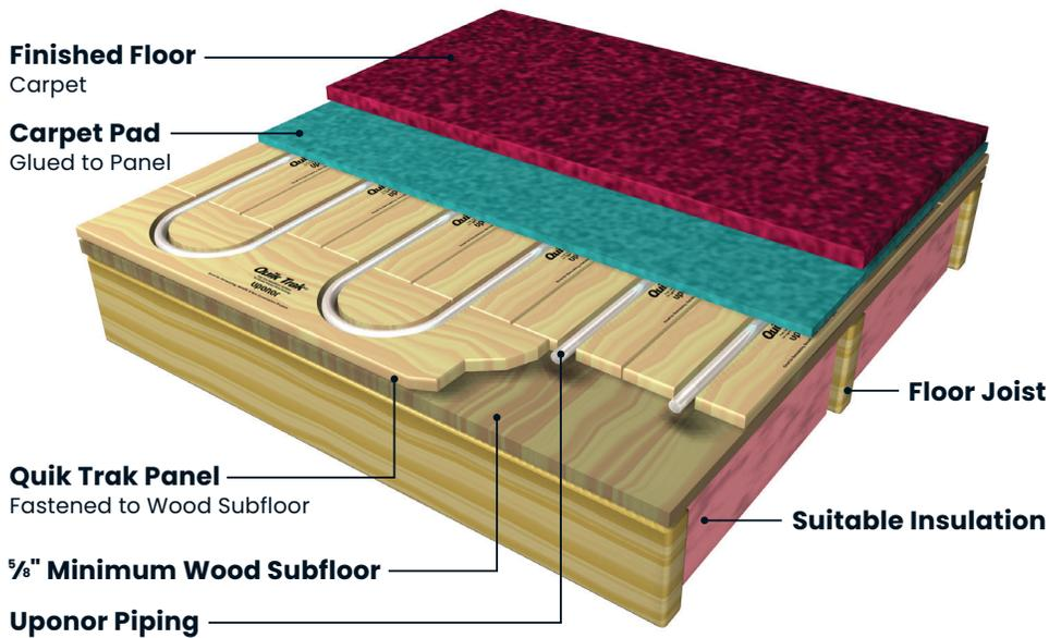
**Figure 6: Quik Trak over a wood subfloor with carpet floor covering**
