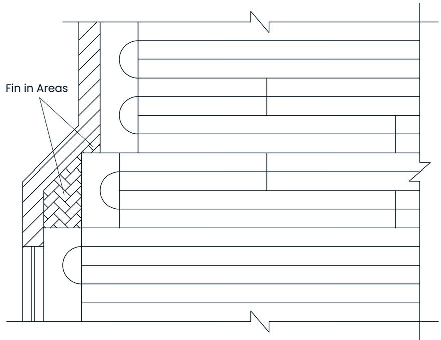
**Figure 23:** When installing the panels in a room with an alcove or bay area, remember to allow enough room for the return panels. Fill any areas not covered with panels with ½" plywood.
