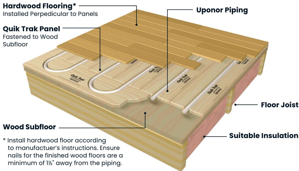
**Figure 4: Quik Trak over a wood subfloor with hardwood floor covering**
