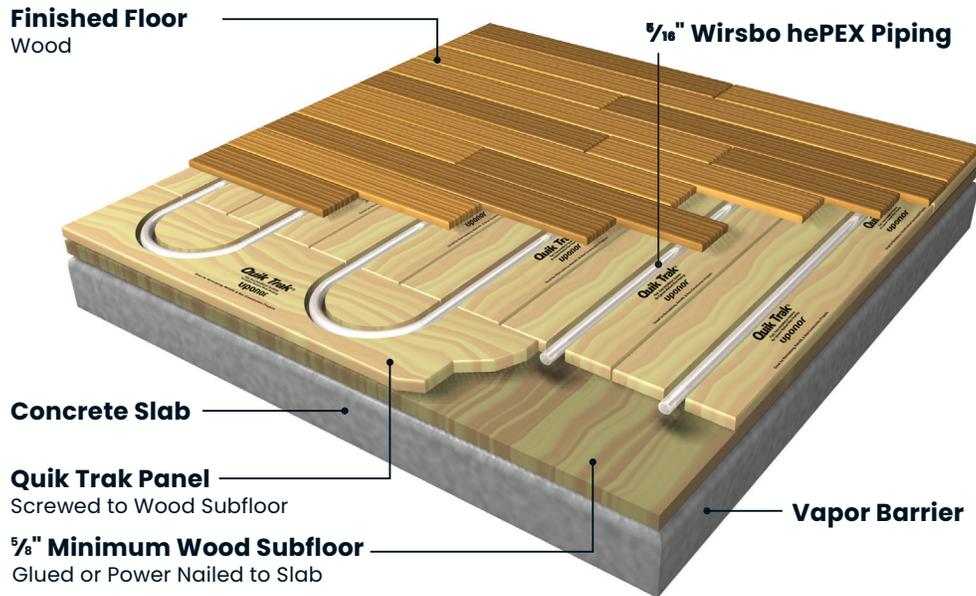
**Figure 7: Quik Trak over an existing concrete slab**
