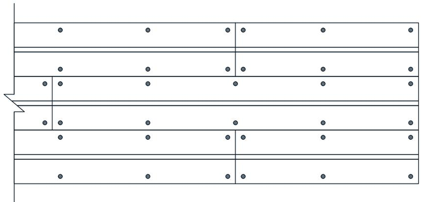
**Figure 20: Fasten panels with 10 screws**
