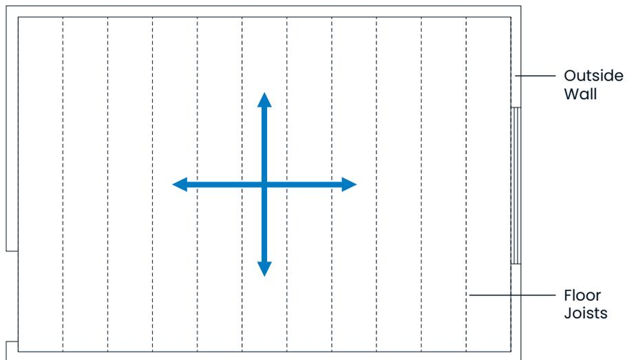
**Figure 16:** For a wood-finished floor covering, install Quik Trak panels perpendicular to the direction of the finished-wood floor boards.
