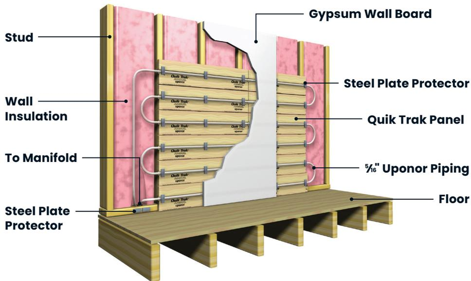
**Figure 8: Quik Trak radiant wall installation**
