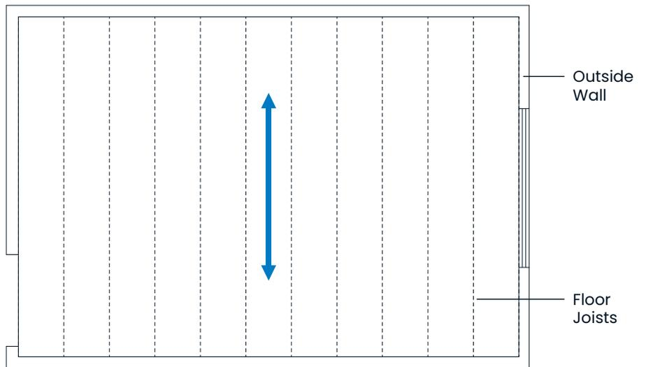
**Figure 15:** For carpeted floors, install Quik Trak panels parallel to the exterior wall to allow the warmest water to reach the coldest area first.
