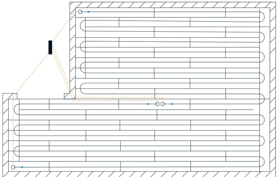
**Figure 13: Manifold location in the joist cavity**
