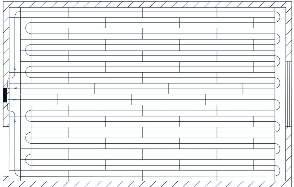
**Figure 10: Manifold location in the wall**
